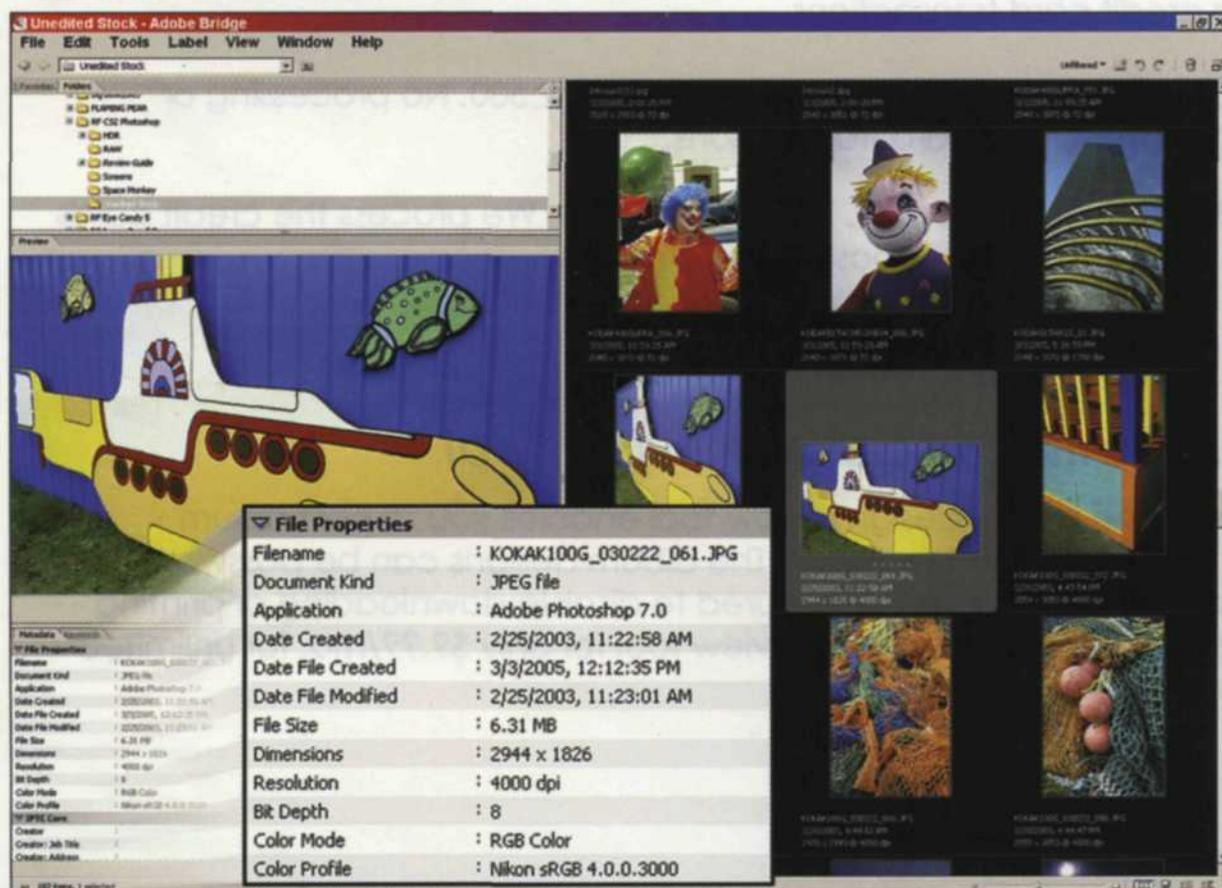
The new CS2 Bridge program works with all new CS2 products and reads a wide variety of file formats from each. The bridge program can be loaded by itself or accessed from inside each CS2 program. Folder directories, upper left; expanded view in left middle; EXIF info in lower left, and thumbnail index at right.
